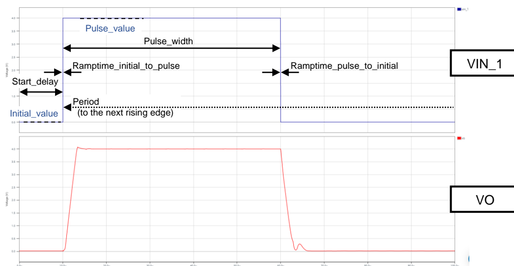
Figure 3. VSOURCE parameters and its waveform
